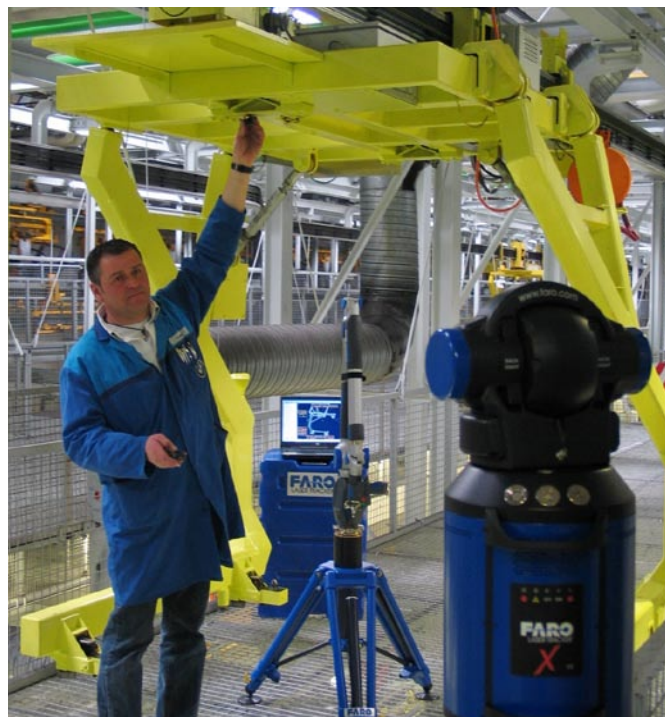
The Track ScanArm is particularly impressive for its mobility when measuring assembly jigs.
