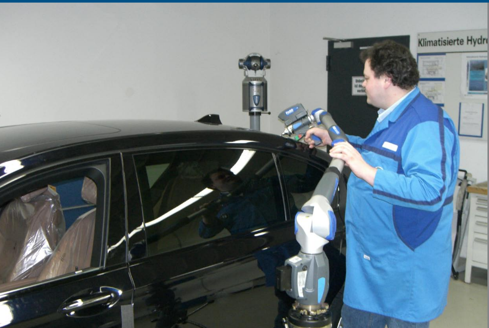
The FARO system is equally impressive for taking exterior as for interior measurements in Dingolfing and Regensburg.
