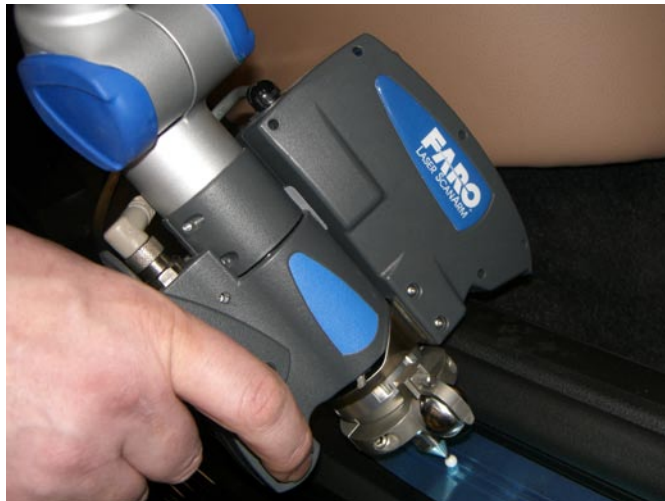
Tactile measurements or the scanning of surfaces are ideal for precisely those places that cannot be reached with the laser tracker.
