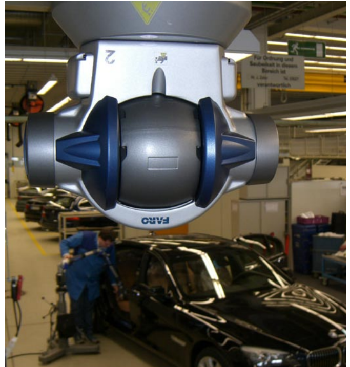
The laser tracker is suspended from the ceiling in Dingolfing. As a result, the possibility of any 'outside contact' can be excluded.
