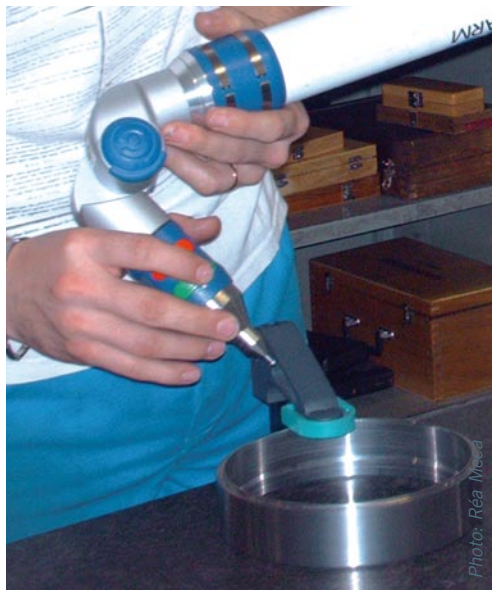
Part inspection with the FaroArm.
