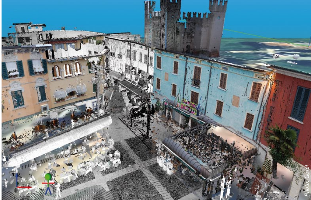
Scan of the historic centre of Sirmione, Italy, taken with the FARO Laser Scanner Photon.
