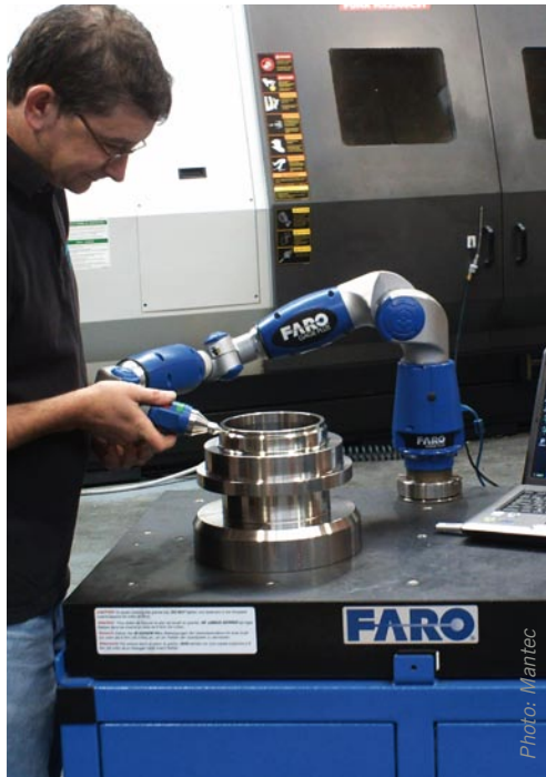
Mantec is using the FARO Gage Plus within their machining facilities to inspect intricate components.
