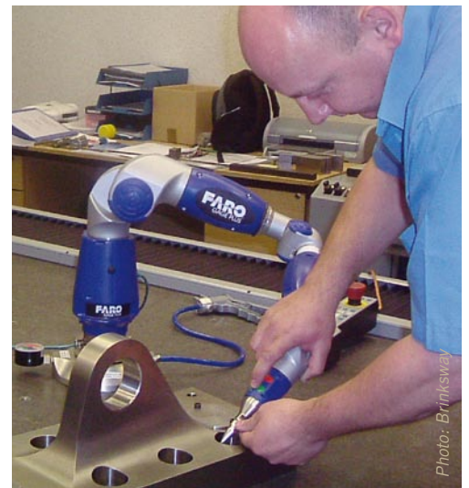
Brinksway Tool use the FARO Gage Plus to inspect Aircraft tooling, jigs and fixtures.
